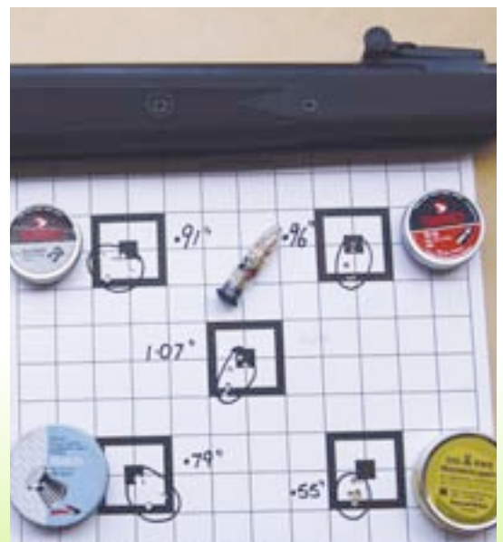
(Right) Hatsan target. We chronographed all the different pellets. The Gamo TS 10 was the slowest and also the heaviest, and the Raptor the lightest and the fastest by far. The speed achieved by each pellet is directly related to their weight. The RWS pellets lived up to their reputation and gave the smallest group.
