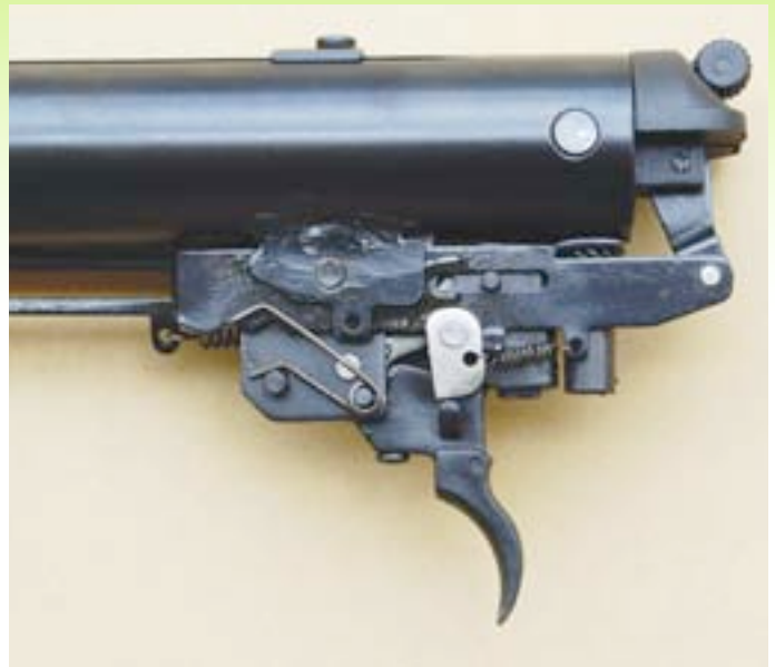
(Above) The trigger assembly of the Hatsan 125. (Right) The automatic safety activation bar which goes all the way from the safety at the rear of the cylinder to the front of the trigger assembly where it is activated by the cocking bar as the rifle is fully cocked. Note that all parts are steel. (Left) The other side of the trigger of the Hatsan.
