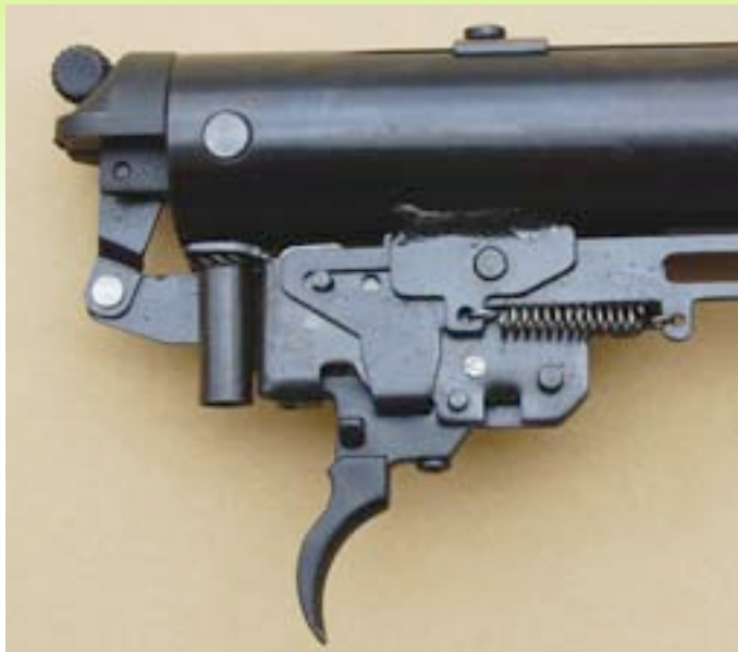
(Above) The trigger assembly of the Hatsan 125. (Right) The automatic safety activation bar which goes all the way from the safety at the rear of the cylinder to the front of the trigger assembly where it is activated by the cocking bar as the rifle is fully cocked. Note that all parts are steel. (Left) The other side of the trigger of the Hatsan.
