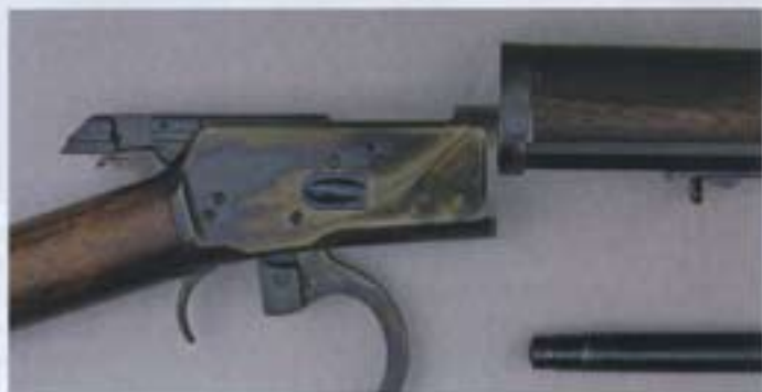
(Above) Barrel reinforce The barrel reinforce can be seen through the top of the action. The threaded hole is where the magazine tube screws into (Above right and right) The action must be open to take the rifle down. The magazine tube is removed and the two major parts simply twist and separate. (Left) Magazine tube end
