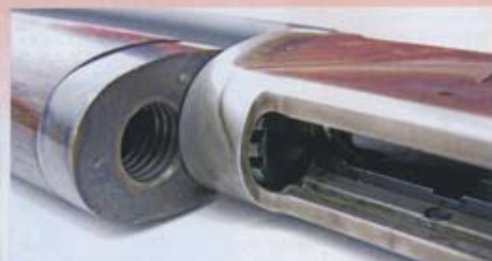
(Above) Barrel reinforce The barrel reinforce can be seen through the top of the action. The threaded hole is where the magazine tube screws into (Above right and right) The action must be open to take the rifle down. The magazine tube is removed and the two major parts simply twist and separate. (Left) Magazine tube end
