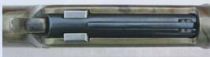
(Left) The lever on the end of the magazine tube hinges out. This is used as a lever to unscrew the magazine tube from the rifle.
