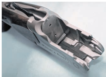
Browning under lug protrudes from bottom of standing breech and dual steel cocking bars slide in recess in bottom of receiver. Barrels are hinged on trunnions.
