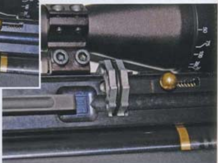
(Above) The magazine fitted into the action. Take particular note of the slot to the back of the magazine which takes the small boss spoken of in the text. (Above inset) Shows the magazine slot in the action with the magazine retaining bolt and the pellet punch which chambers the pellet and remains in place during the firing process.
