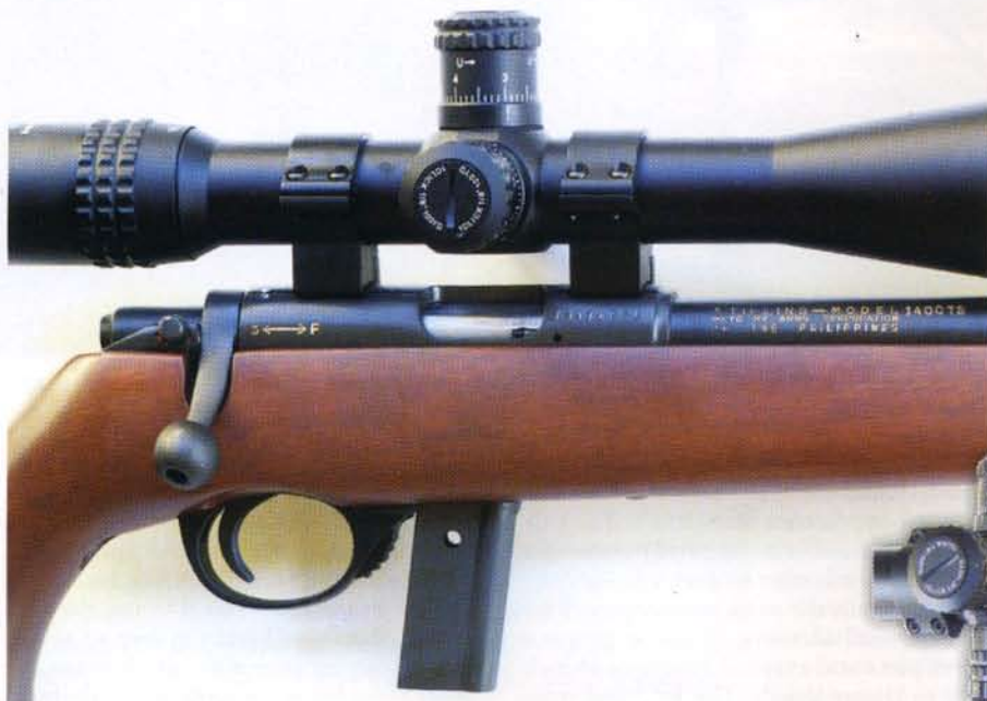
LEFT: The 1400's receiver is grooved for dovetail mounts. The safety is located immediately behind the bolt and the rifle comes with a 10-shot magazine.
